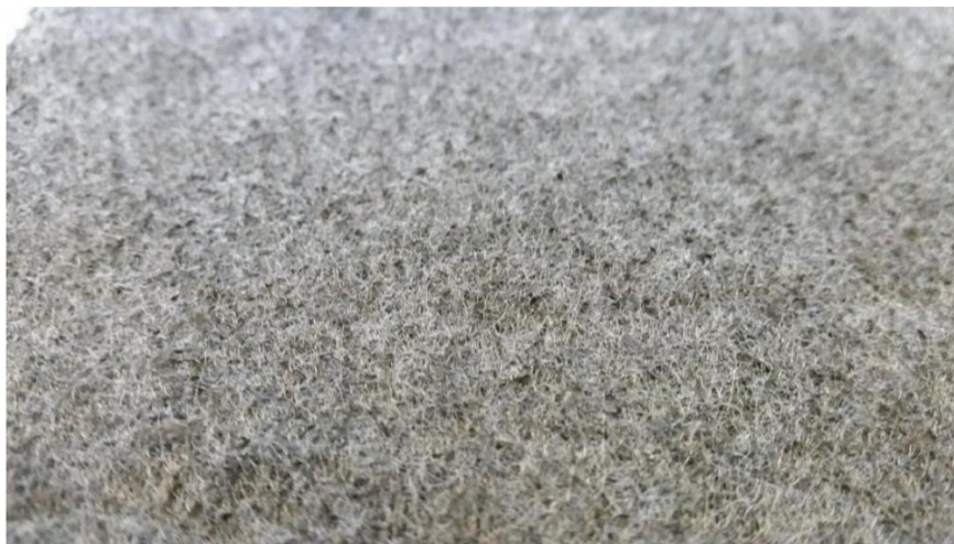
Polyester septum impregnated with activated carbon powder
